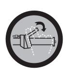
The throttle controls your speed and the steering wheel or handlebars move the jet thrust nozzle in different directions to steer the boat. Do not decrease throttle when trying to steer, and always remember that boats don't have brakes.
