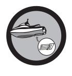
Items such as long hair, loose clothing or life jacket straps can become entangled in moving parts within the water intake grate and cause severe injury or drowning. Stay away from the intake grate.
