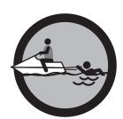
Do not apply throttle when anyone is at the rear of the boat. Water forced from the jet thrust nozzle can cause serious bodily injury.
