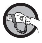
Securely attach the engine shut-off cord (lanyard) to your wrist or life jacket and wear it at all times. This will ensure the engine stops should you fall overboard.
